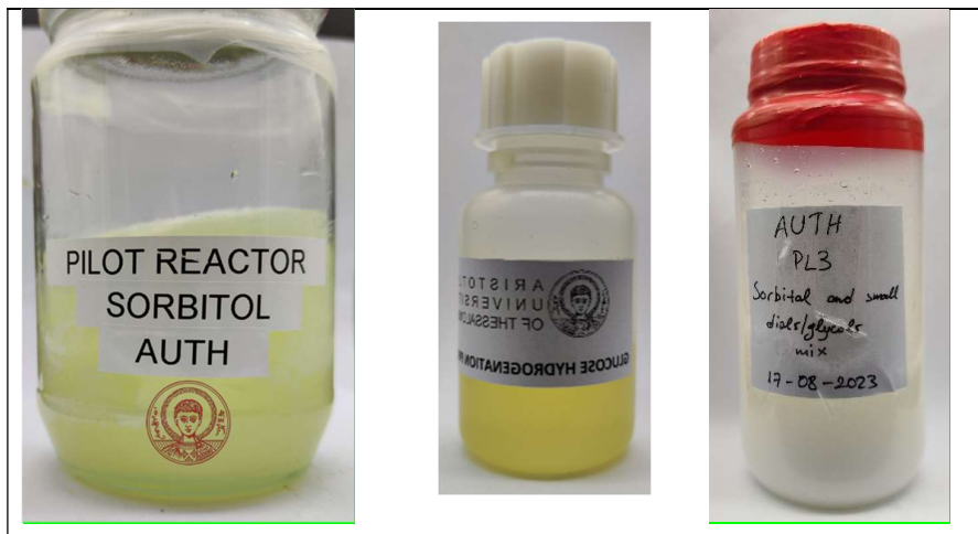
Figure 13. Pilot scale (left) and small scale (middle) sorbitol product from glucose hydrogenation and the sorbitol/EG/GLY/1,2-PDO product mixture produced from glucose hydrogenolysis (right).
