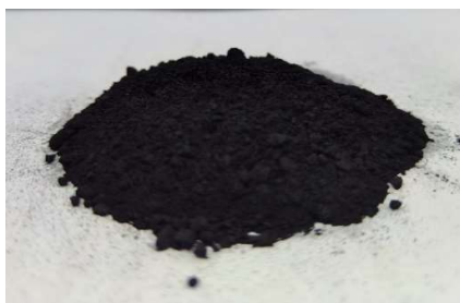
Figure 8. Picture of the 5% Ru/AC catalyst produced at AUTH (PL3)
