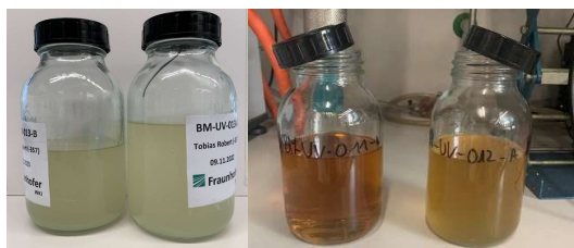
Figure 18. Resins derived from sorbitol (left) and succinic acid (right).
