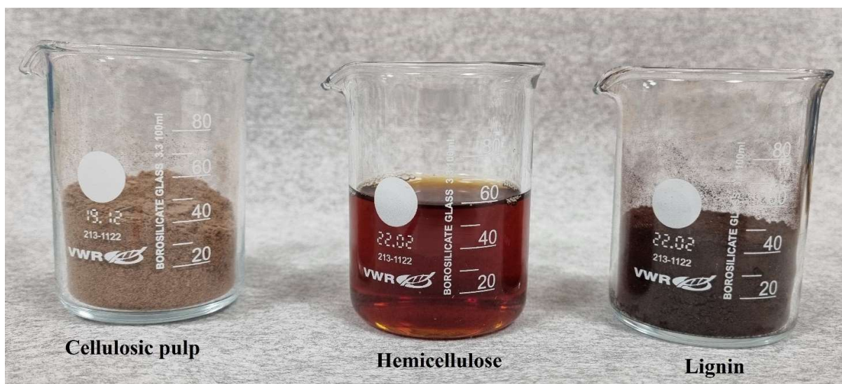
Figure 4. Cellulosic pulp, hemicellulose and lignin isolated from hardwood sawdust.
