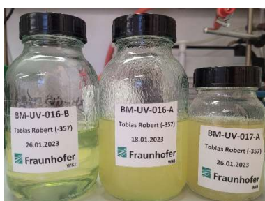
Figure 19. Resins obtained from experiments with nanocellulose, reference left, with pulp in the middle, nanocellulose on the right.
